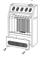
Figure 6 - Removing Front Panel of Heater
